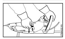
• Release the trigger switch (1) and the switch lever (2).
