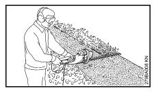
To extend your reach, hold the control handle with one hand and operate the auxiliary switch at the rear of the control handle with the other hand.
