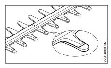
The blades are covered by the blade guard in the idle position.
