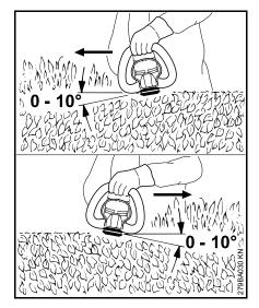
Hold the cutting blade at an angle of  $0^{\circ}$  to  $10^{\circ}$  as you swing the hedge trimmer horizontally, using both sides of the blade.
