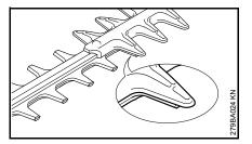
The blades are partly covered by the blade guard in the idle position.
