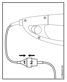
Insert the plug (1) into the extension cord coupling (2).
