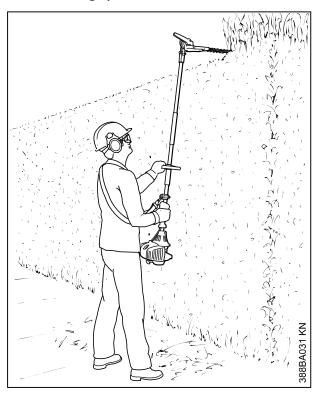
Hold the hedge trimmer vertically and swing it in an arc to make maximum use of its reach.
