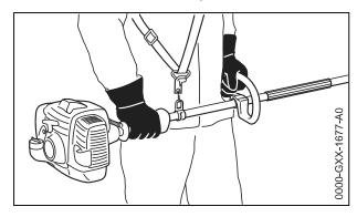
Right hand on control handle, left hand on loop handle on the shaft, even if you are left-handed. Wrap your fingers and thumbs around the handles.
