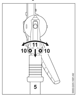
► Loosen the clamp screws (10).
