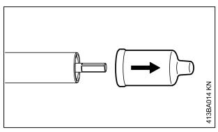
Pull the protective cap off the end of the drive tube and keep it in a safe place.
