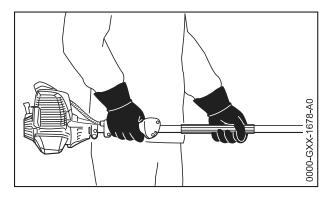
Right hand on control handle, left hand on handle hose on drive tube, even if you are left-handed. Wrap your fingers and thumbs around the handles.
