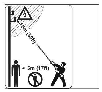
Do not allow anyone within 5 meters of your position – **risk of injury** by moving cutting blades or falling cuttings! This distance must also be maintained in relation to objects (vehicles, window panes) – **risk of property damage!**
