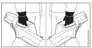
► Hold and guide the blower by the control handle with one hand, wrapping your thumb around the control handle.
