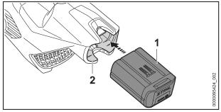
► Insert the battery (1) into the battery compartment (2) as far as it will go.
